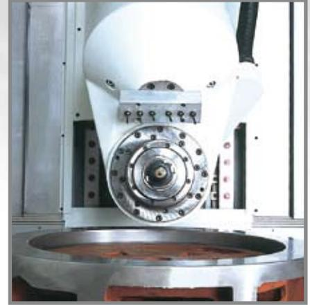
► The latest technology torque motor manages the B axis continuous swivel milling head , it guarantees maximum movement dynamic and linearity and thanks to the absence of those traditional mechanical kinematics parts, it results a much higher performance on finishing surface. The direct reading system by a high precision angular encoder is being integrated for maximum precision.
